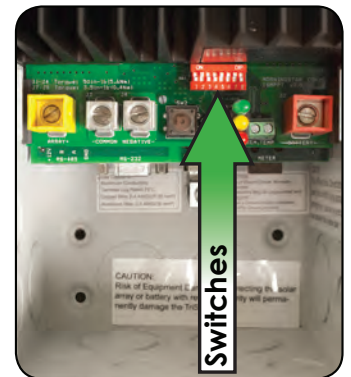
Morningstar Charger with Wiring Box Cover Removed.
