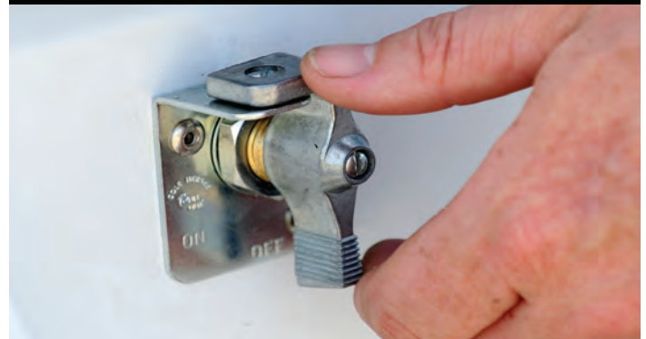
Figure 15: Main Battery Disconnect in the OFF position
