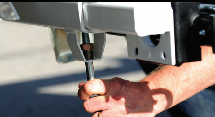
Figure 9: Outrigger Sleeve Locking Pin
