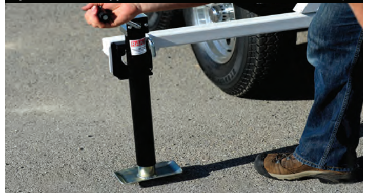
Figure 10: : Outrigger Arm Extended & Jack Stand Deployed
